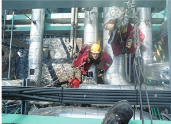
**Figure 2. Using handheld XRF analyzers, an inspector conducts rope access PMI at a Canadian refinery.**
